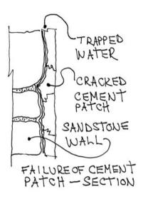
Other defects include pieces of sandstone falling away from the underside of cornices, lintels and other blocks that project from the wall. Facing up in cement mortar is a common response but, for the reasons just described, it is not a proper repair.
