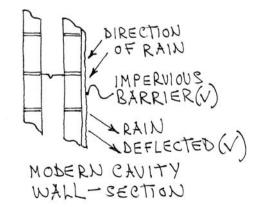
A cavity wall is designed to keep water out by presenting an impervious barrier to the weather. It is for that reason dense
