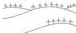
Multiple windfarms relate to same characteristic, to create consistent image and reinforce perceived appropriateness of each windfarm. However, by occupying every incidence of specific characteristic, will become key characteristic that changes overriding character
