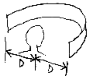
Figure B14: A cylindrical panorama can be superimposed on the scene when viewed from the centre of curvature of a curved surface whose radius is the correct viewing distance.
