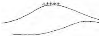
Windfarm appears as minor feature, both horizontally and vertically in relation to the surrounding landscape
