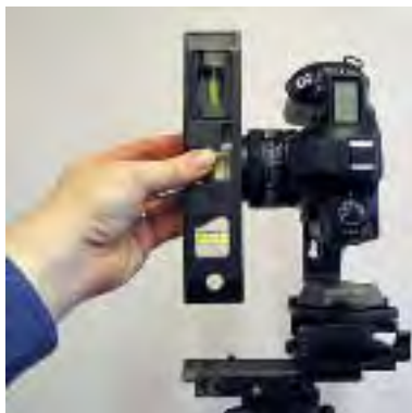
Figure E4: Placing a spirit level against the filter-ring of the camera lens allows the camera to be levelled accurately. This works both for landscape and portrait orientations of the camera.
