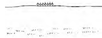
One option is to cluster wind turbines close together upon a local area of flatter ground, so that the variation is less obvious than the image of a single collective feature
