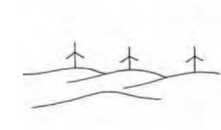
Wind turbines relate to small scale undulations at a local level. However, if the key views are distant, these undulations would not be obvious and the wind turbines would alternatively appear in closest association with the broad scale landform
