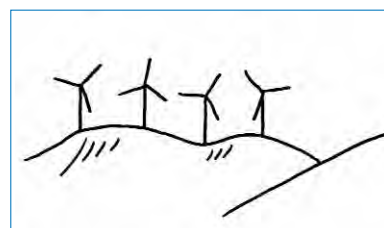
Sketches 3 and 4: A double line of turbines hides the profile of a ridge, while a single line relates to it.
