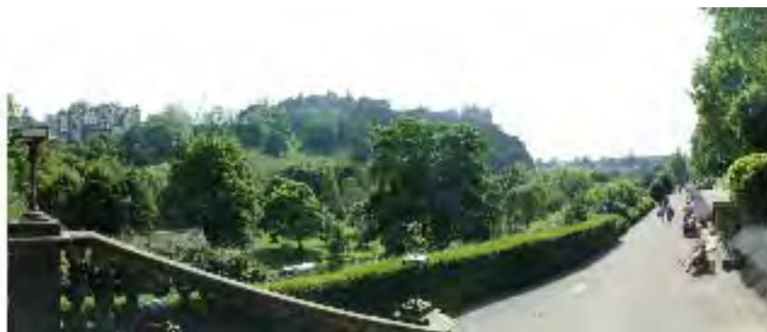
Figure B17: Cylindrical panorama with a horizontal field of view of 106^\circ . This is the type of image produced by a rotating lens panoramic camera or by splicing together single frames from a conventional panorama. The horizontal scale is the same across the whole width of the image. The viewing distances for both panoramas are the same, so the scales are equal in the centre of the planar panorama.
