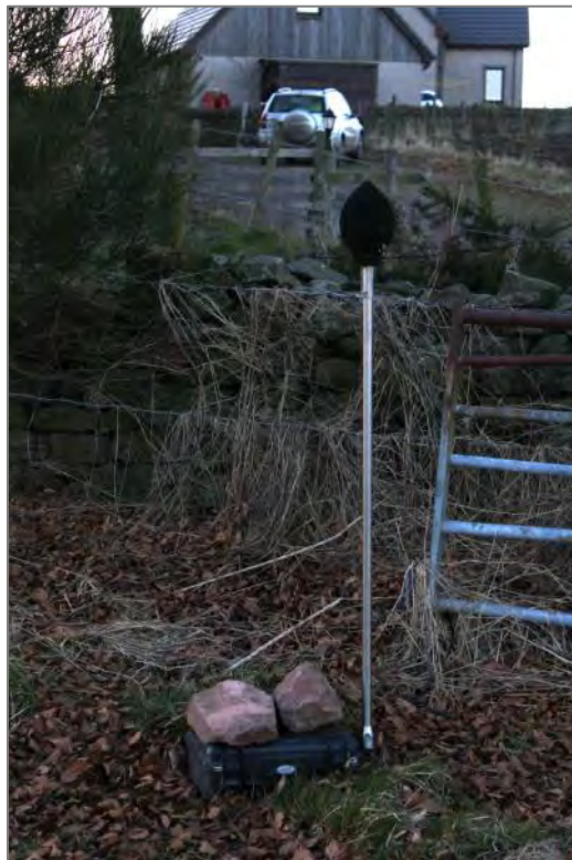
Figure 8.5 – Noise monitoring kit at position 2 looking northeast toward Scotia House.
