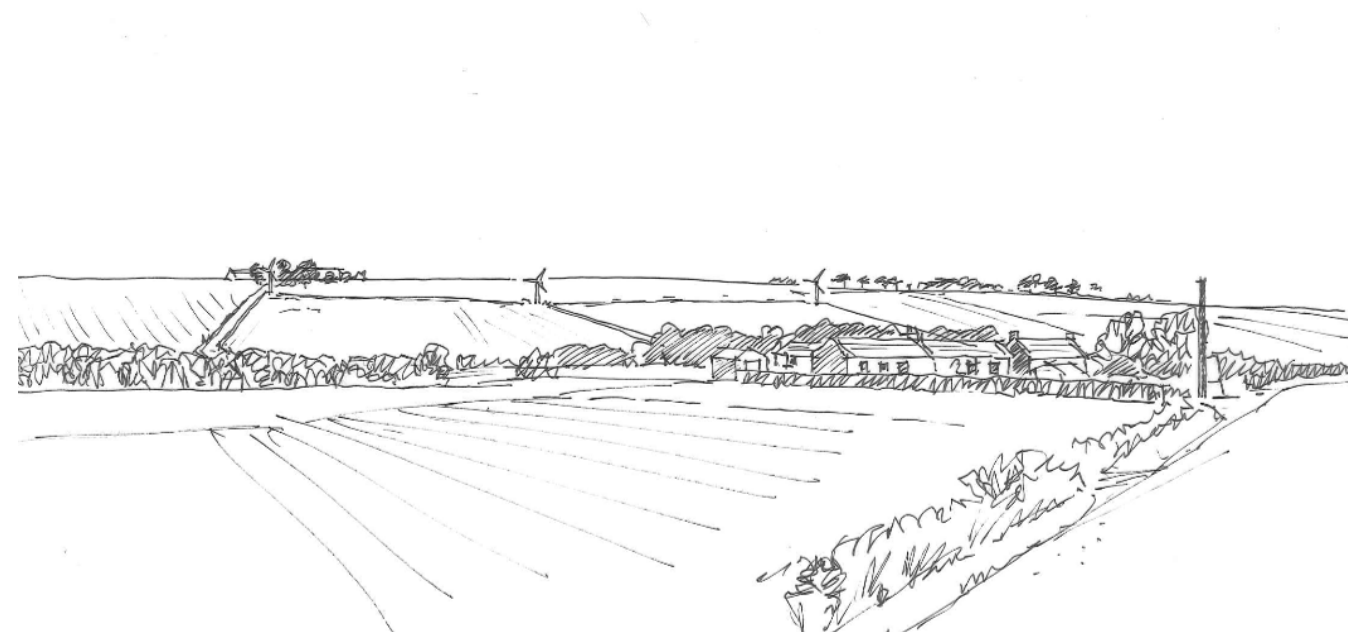
Lunan Water Valley: Small/medium (15-30m high) turbines do not dominate the modest valley slope and blade tips can be aligned with trees and buildings on the horizon
