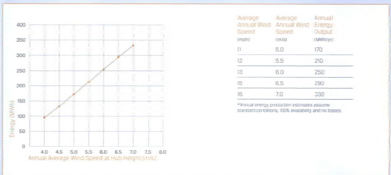
Annual Energy Production*: 24-Meter Rotor Standard Air Density, Rayleigh Wind Speed Distribution
