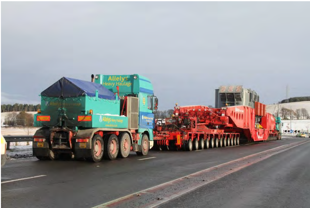
Rear tractor unit in use on abnormal load move
