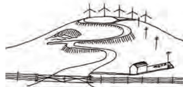
Insensitive siting and design of windfarm infrastructure creates complex image and conflicts with underlying landscape character
