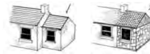
extension and poor use. The good example incorporates a technique that is highly recommended and helps to conceal the joints between old and new where side extensions are involved and that is a slight set back from the house front.
