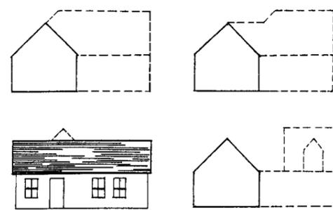
to demonstrate (e.g. by perspective sketches) that the roof of the extension is not readily viewed above the roofline of the original building.
