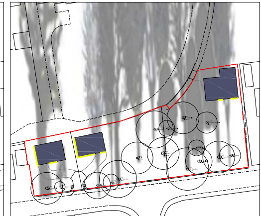
NOON Plot 1- 34% of South Elevation & 100% of West in direct sunlight Plot 2- 81% of South Elevation & 100% of West Elevation in direct sunlight Plot 3- 43% of South Elevation in direct sunlight
