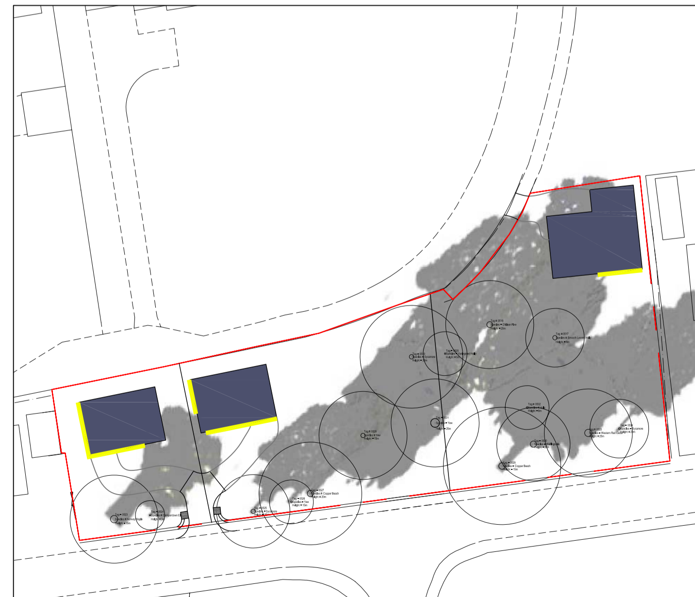
3PM Plot 1- 73% of South Elevation & 100% of West Elevation in direct sunlight Plot 2- 94% of South Elevation & 63% of West Elevation in direct sunlight Plot 3- 50% of South Elevation in direct sunlight
