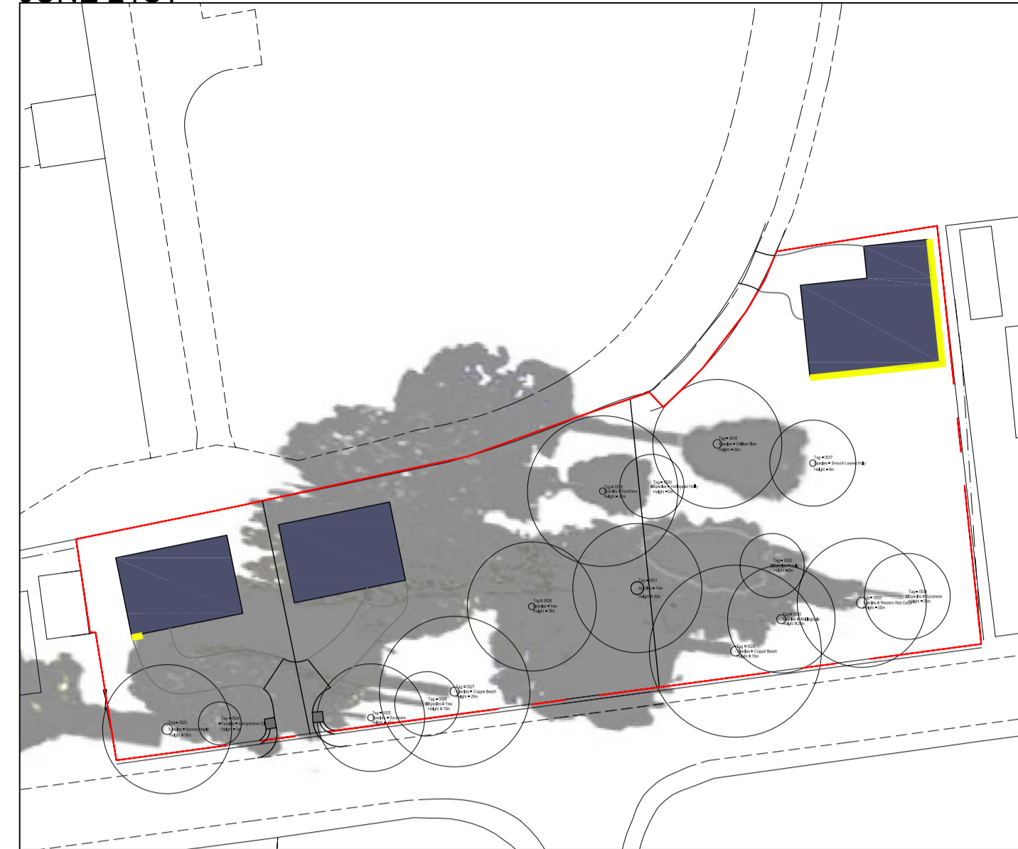
9AM Plot 1- 9% of South Elevation in direct sunlight Plot 2- Not in direct sunlight Plot 3- 100% of South Elevation & 100% of East Elevation in direct sunlight
