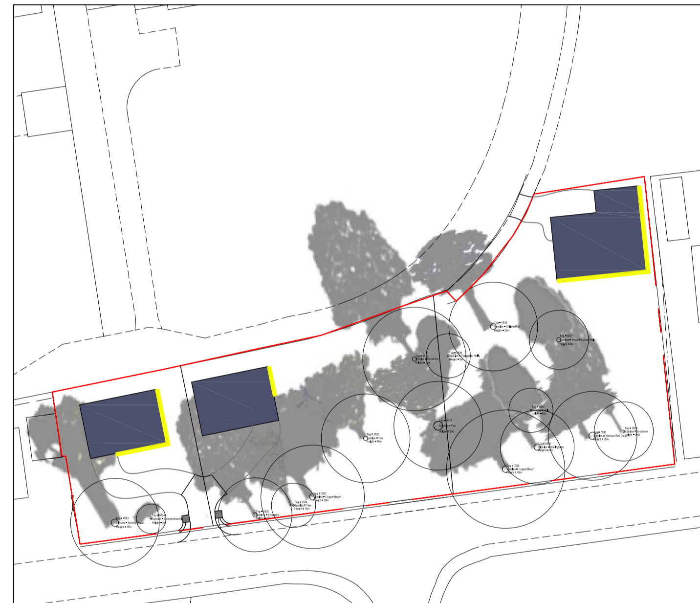
NOON Plot 1- 66% of South Elevation & 100% of East in direct sunlight Plot 2- 55% of East Elevation in direct sunlight Plot 3- 100% of South Elevation & 100% of East Elevation in direct sunlight
