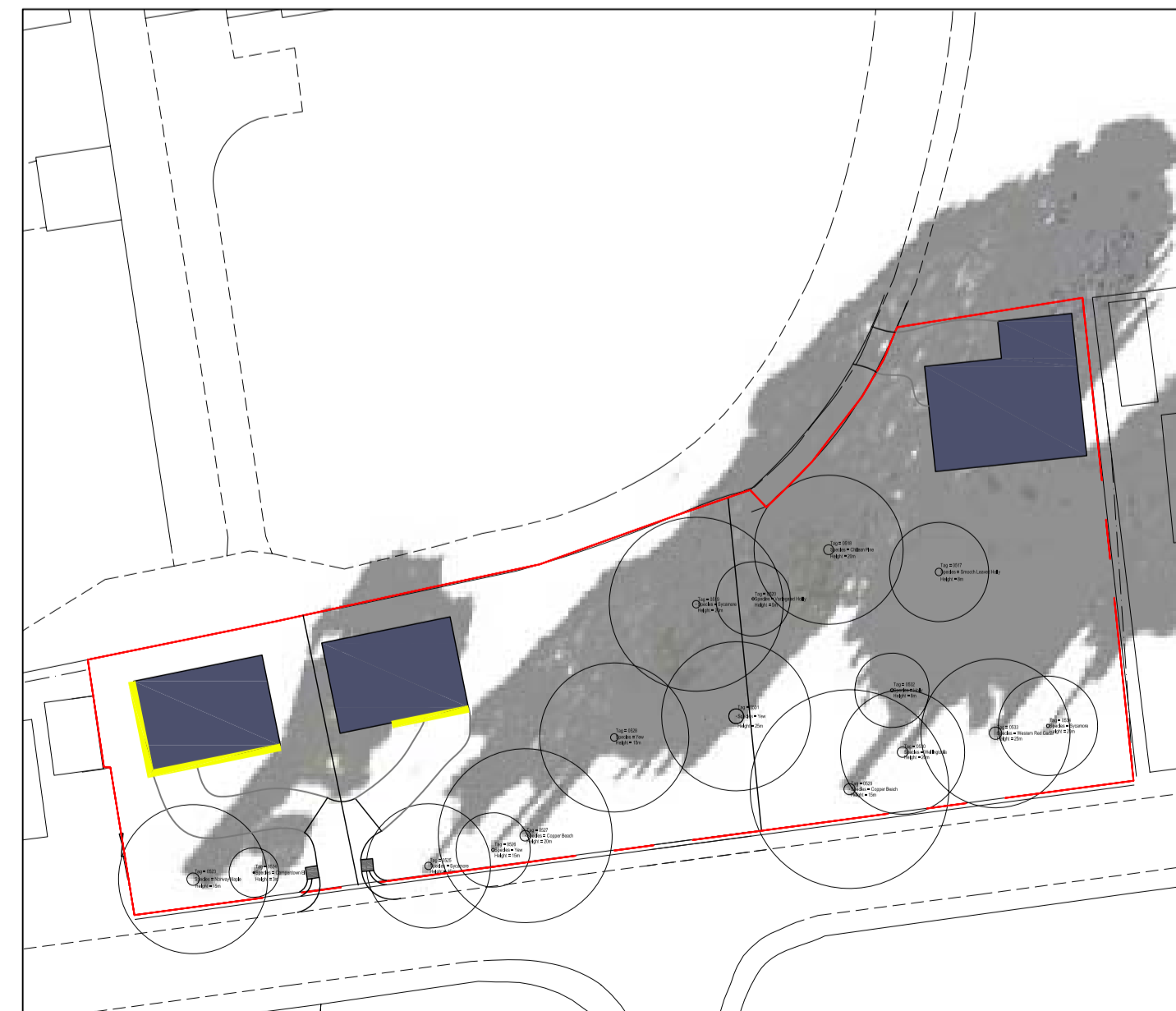
3PM Plot 1- 100% of South Elevation & 100% of West Elevation in direct sunlight Plot 2- 60% of South Elevation in direct sunlight Plot 3- Not in direct sunlight
