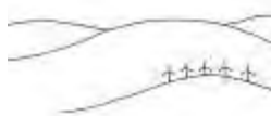
Individual wind farm relates directly to landform characteristic as single line upon horizon
