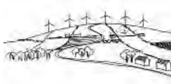
Visual link between wind farm and elements of known size, aid perception of scale and distance, emphasising the height of the wind turbines
