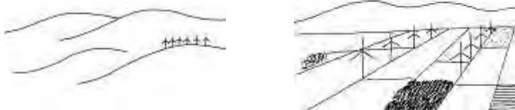
A wind farm layout appears simplest where it relates directly to the underlying landscape characteristics
