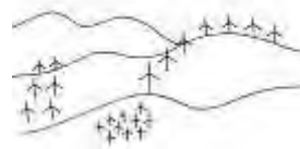
Although no clear area of space between wind farm groups, distinction highlighted due to contrasts of turbine scale and layout (variety of development type creates visual complexity).
