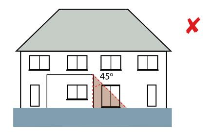
The shape formed by the 45° line encloses the centre of the window on the adjacent neighbouring property which ensures that the level of daylight received by that window is adversely affected.
