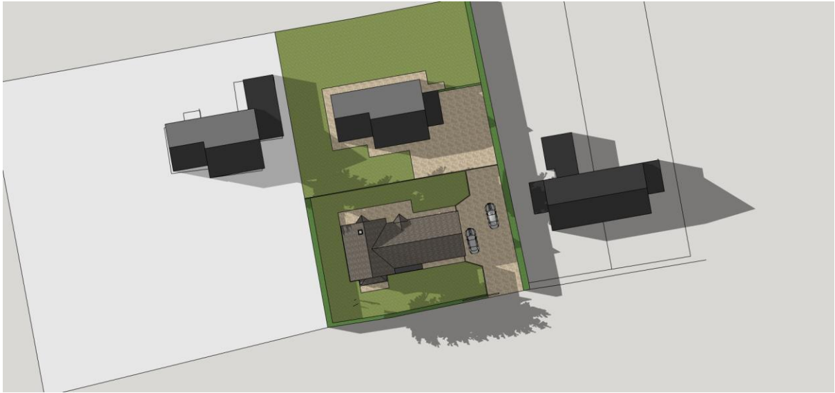
Sun path on the equinox in the afternoon. Once again, there is no impact on the surrounding houses caused by this new house.
