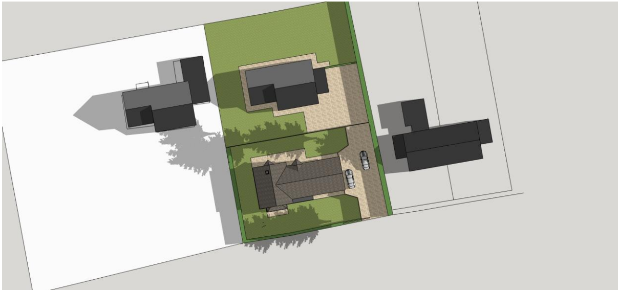
Sun path on the equinox in the morning. The proposed house makes no impact on the surrounding houses.
