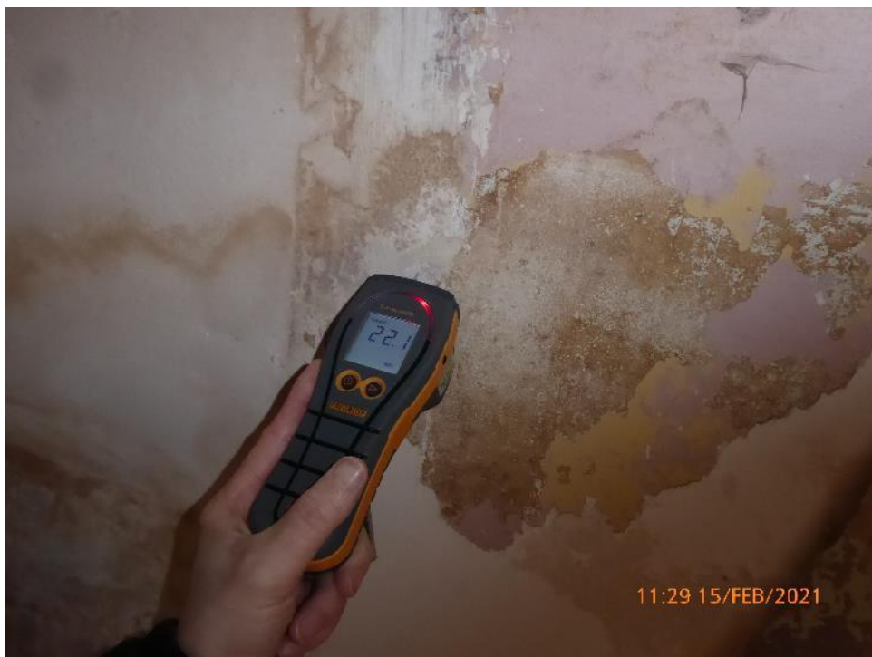
31. High moisture meter readings within attic
