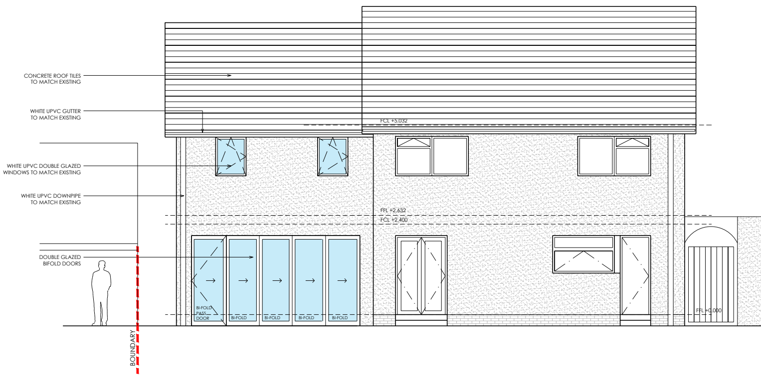
03 PROPOSED EAST ELEVATION SCALE 1:50
