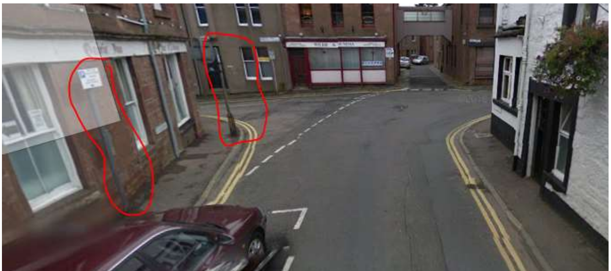
Image 11: Remove poles and place signage on building. If appropriate to replace then consider either galvanised or black.
