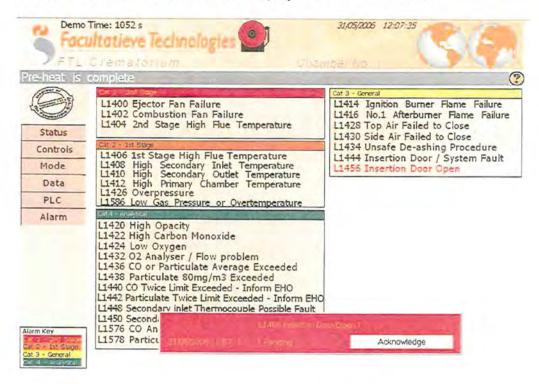
The alarms are grouped into categories due to their relevant severity. This is to make fault finding by an operator an easier task.
