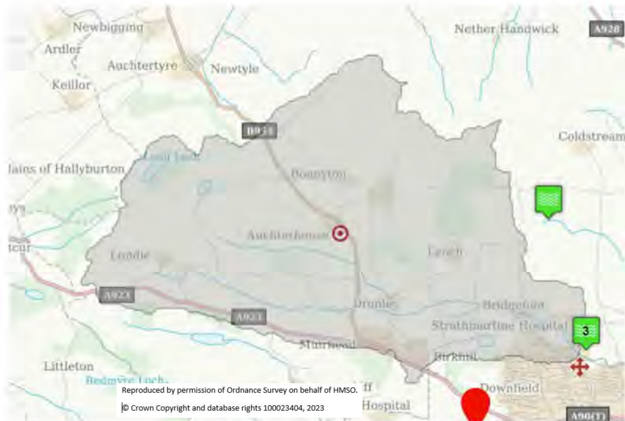
Figure 5 – Dighty Water catchment at Hawthorn Cottage, as defined by the FEH Web Service (FEH Web Service, 2021)
