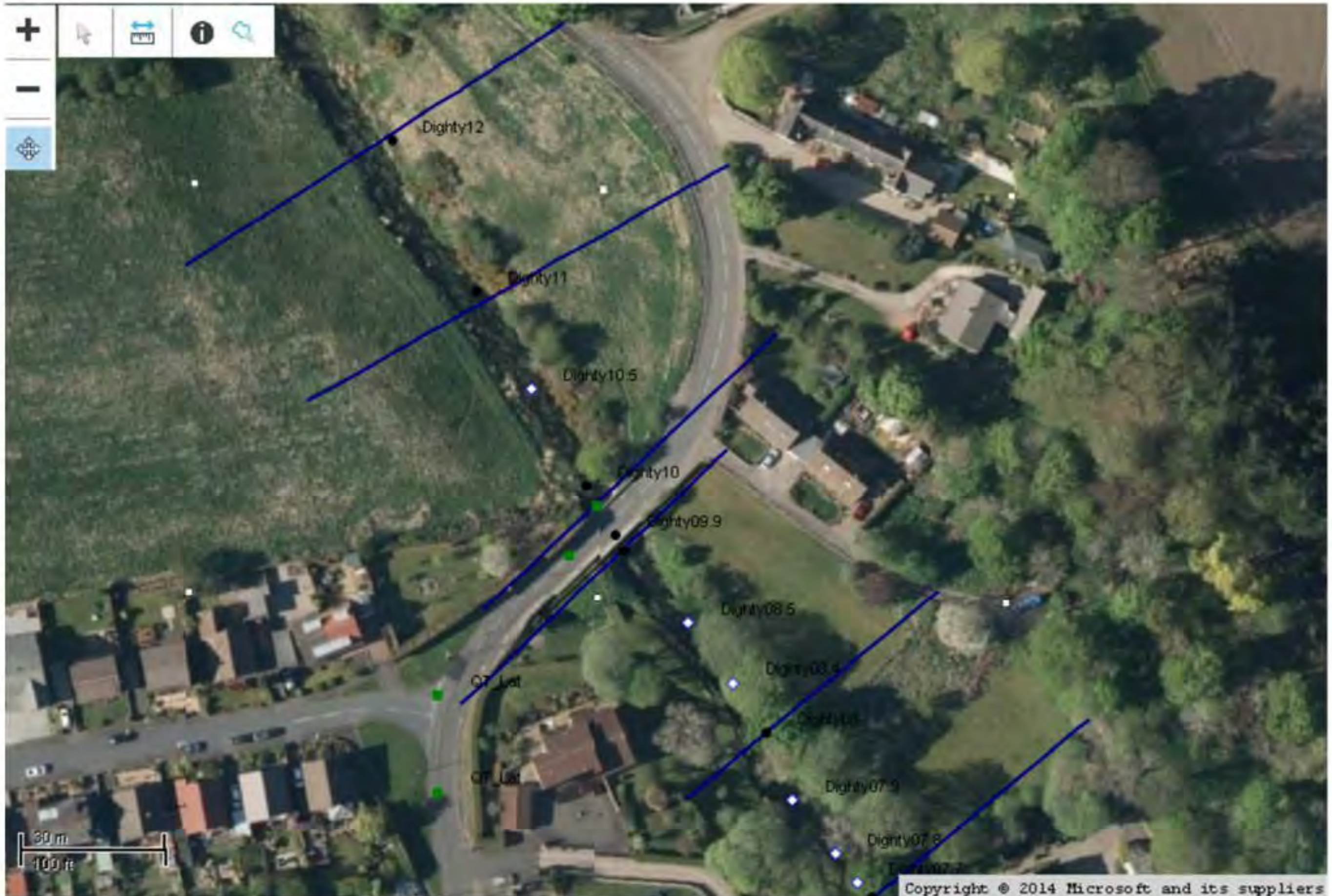
Figure 7 – Cross section locations (1 of 3)
