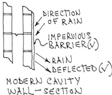
A cavity wall is designed to keep water out by presenting an impervious barrier to the weather. It is for that reason dense
