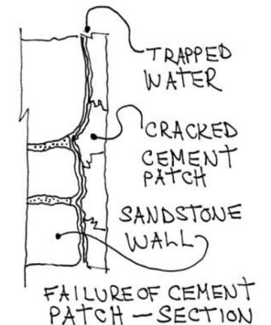
Other defects include pieces of sandstone falling away from the underside of cornices, lintels and other blocks that project from the wall. Facing up in cement mortar is a common response but, for the reasons just described, it is not a proper repair.
